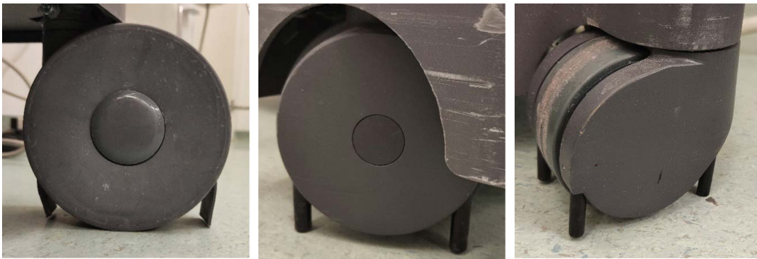
Figure 1: Wheels of mobile X-ray machines, showing cable deflectors, at front and back of all castors, and reaching fully to the ground.
