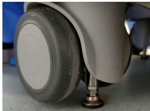
Figure 3: Wheel shroud on an operating table, showing incomplete deflection protection (metal post is deployed table brake, which retracts when table is to be moved)
