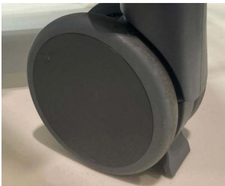
Figure 2: Wheel of Mindray A9 anaesthesia workstation, showing cable deflector on leading edge
